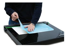
2 Remove the release paper on the cover and smooth down the printed cover sheet, starting from the left and moving to the right.
