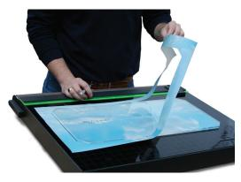
Trim the printed cover sheet using the ImageBack template at the desired size.
