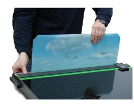
3 Fold in the outside edges of the cover wrap to attach to the edges of the inside cover. Push the cover into the pinch roller to adhere the edges.
