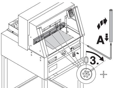
With the special wrench (A) the 3 eccentrics should be screwed down (3.) until the paper is cut along the entire length of the blade
