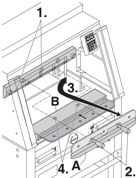
Remove 2 blade screws IDEAL 4860 and 3 blade screws IDEAL 5260, IDEAL 6660 (1.). Loosen the grips (2.) of the blade changing tool (A) lightly and allow the blade to be taken downwards out of the machine (3.). Place the blade into the blade carrier (B) and screw it into place (4.).
