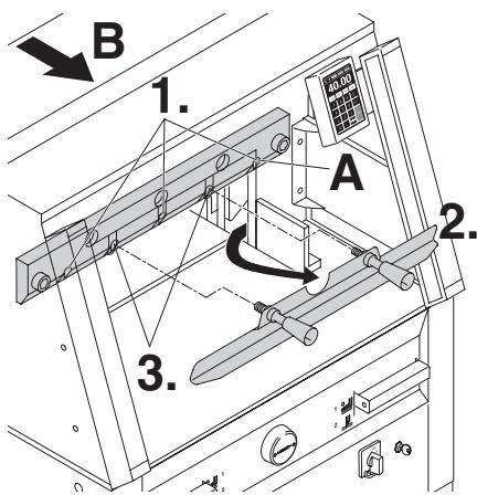
Lightly tighten 3 (IDEAL 4860 has 2) of the 5 blade screws with washers (1.). Remove the blade changing tool (2.). Lightly tighten the remaining blade screws with washers (3.). Return blade changing tool to tool holder (B).
