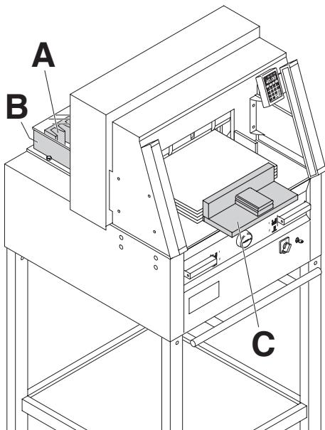
Position the paper on the backgauge (**A**) and side lays left or right (**B**).
