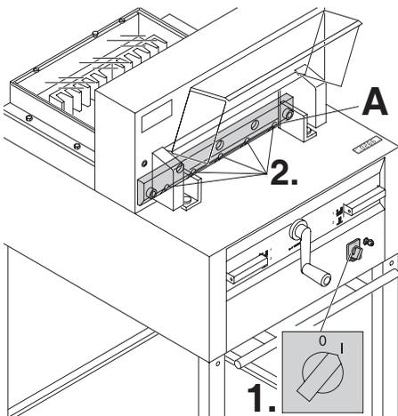
Tighten the blade screws (A) on the right hand side.
