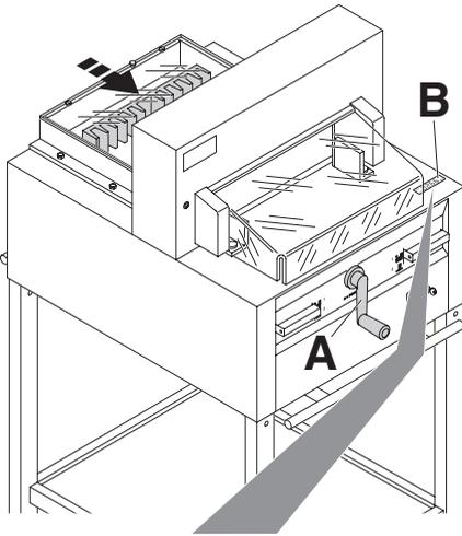
The measurement is set with the backgauge crank. (A) The symbol – rotary direction –  $\rightarrow$  moves to the right on the display (B) (see picture C). The rotary direction of the backgauge crank (A) is indicated on the right. Keep turning the backgauge crank to the right until a measurement appears (see picture E). The reference position is reached. The cutting size can now be set with the handle (A).
