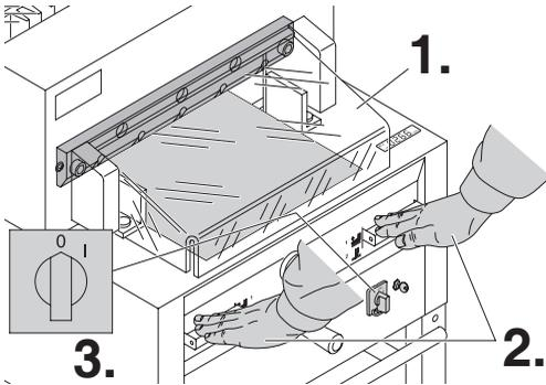
Close the safety guard (1.) Lower the blade by pressing both cutting buttons (2.). Keep one button pressed and turn off the main switch (3.).
