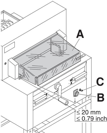
Before working with the machine and after every blade replacement the automatic cut-off function of safety guard (A), (correct if distance between cover and table is  $< 20 \text{ mm}$ ) main switch (B) and control panel (C) must be checked.
