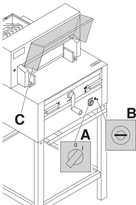
Position the main switch ④ to "I" (**A**). Insert the key ⑥ for the control system and move it to the right (**B**). Open the safety guard ⑩ (**C**). The machine is now ready for use.
