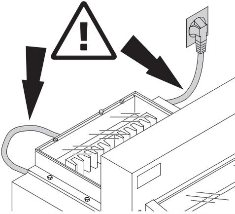
Connect the power cord to a single phase socket.
