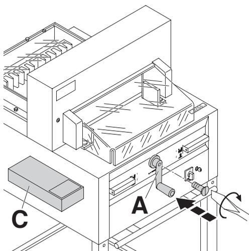
Tighten the backgauge crank (A). Parts and tools are in the tool set (C).
