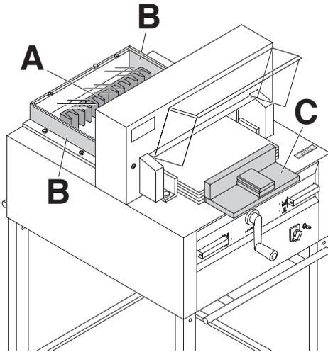
Position the paper on the backgauge (A) and side lays left or right (B).
