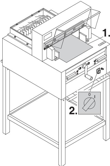
Remove all tools and distribute paper along the entire cutting length (1.). Turn main switch to position "I" (2.).
