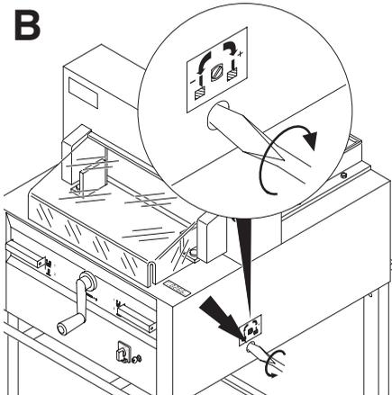
**Poor cutting quality or blade stays in the paper stack.**
