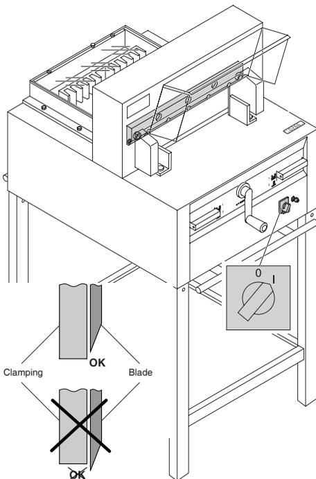
Remove the special wrench and turn on the main switch until the blade returns to the home position.
