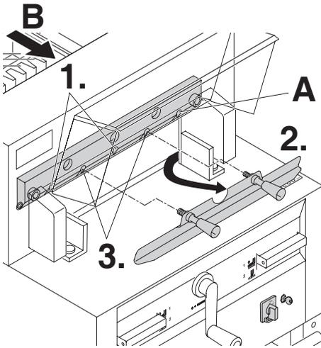
Lightly tighten 2 of the 5 blade screws with washers (1.). Remove the blade changing tool (2.). Lightly tighten the remaining blade screws with washers (3.). Lightly screw in the right blade screw with the washer (A) when the blade is lowered.
