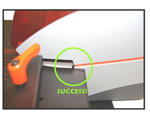
4. Check under the stitcher to make sure that the central rubber foot is aligned with the hole on the bottom of the table. Your Silver Strike Prime Stitcher is now securely assembled; straighten the aluminum backstops, plug in the foot pedal and power supply and happy stitching!
