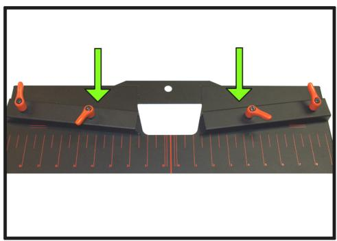
2. Check your stitcher unit and make sure the built-in depth lever is pushed all the way back to the 5" mark. Take note of the two pegs extending from the table; these will fit in the grooves of the stitcher and hold it in place.
